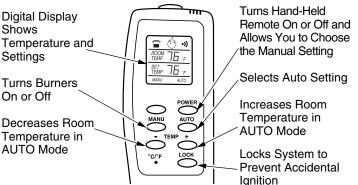
Figure 62 - Thermostat Hand-Held Remote Control Unit (C)GHRCTB
